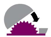
For example, a table saw has a cutting blade at the point of operation. If the saw has a fixed guard to provide protection, then failure of the guard would allow for injury at the point of operation. This might occur if the guard was removed for maintenance, to improve productivity, or if it broke.
